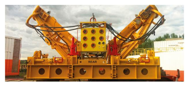
This operation is carried out by using a subsea piling support frame, like our Fast Frame with full levelling capability, to allow the conductor to be installed with a subsea piling hammer rather than a drilling or jetting solution. The subsea piling frame is landed on location and hydraulically levelled by WROV to ensure the vertical tolerances are in specification prior to the deployment of the pre-assembled conductor stack.
