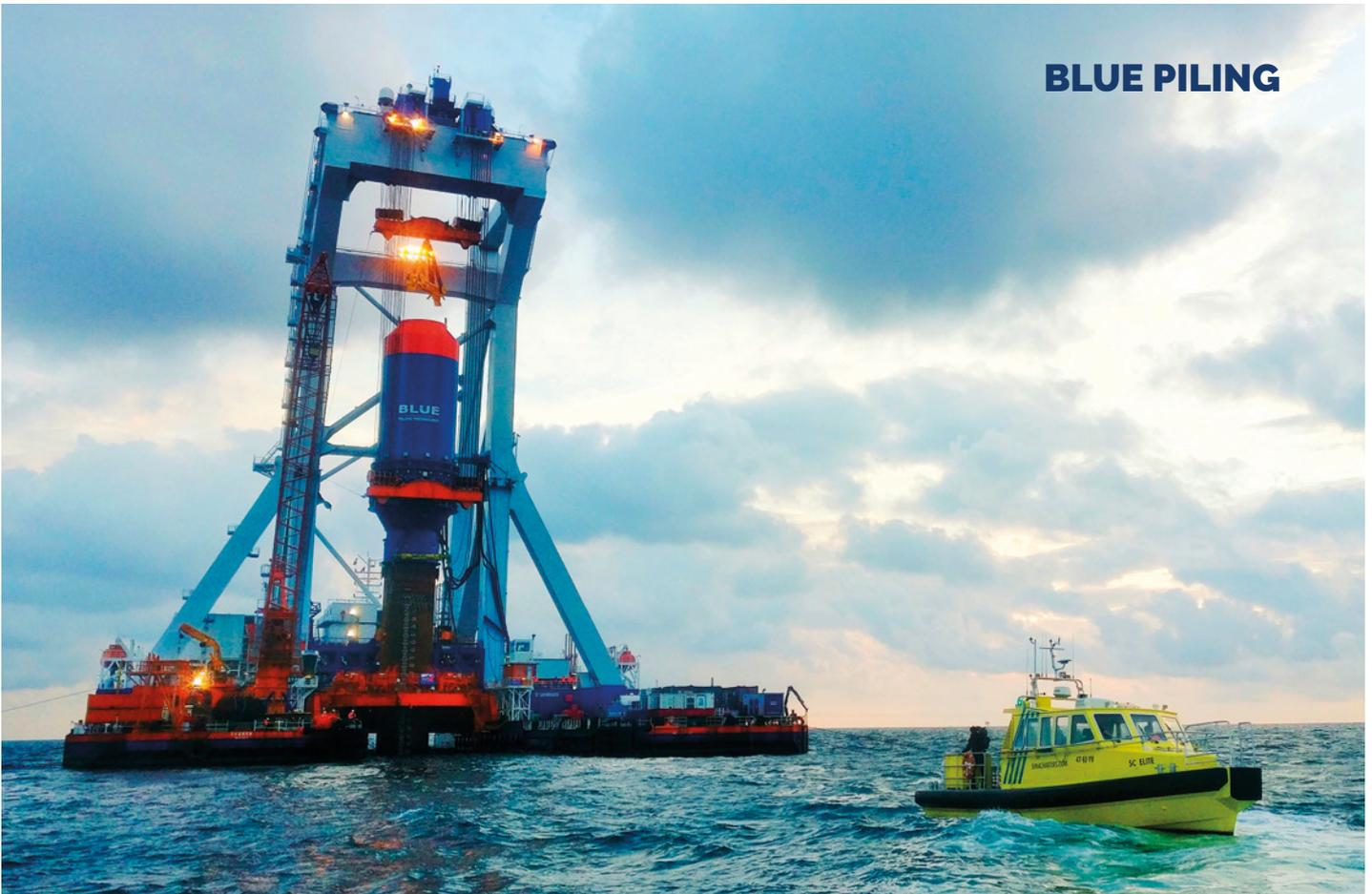
BLUE Piling Technology™ (patent pending) uses the impact of a large (water) mass to drive down monopiles. The BLUE Piling blows aims at silent installation of the next generation monopiles. Unique BLUE Piling Technology features:
